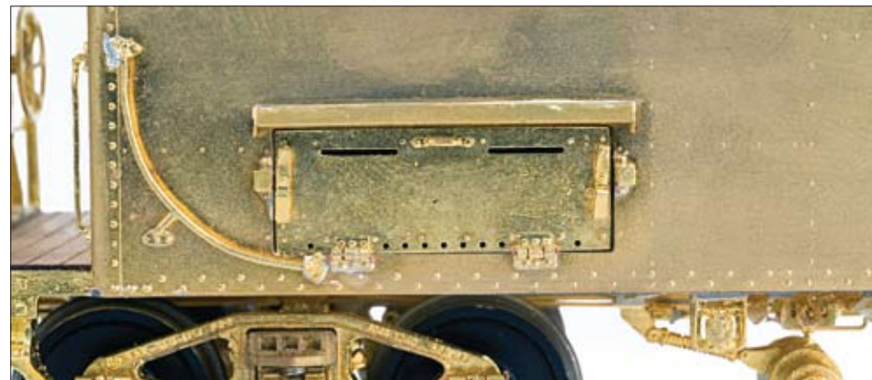
Part of the extra detail required for a trainphone equipped 'cab' is the battery box shown above, it opens and is complete with locking latches on either side. Below is our PRR 2A-F4 type truck that is used a specific versions of the N5 w/cp, note the raised cast lettering on the side frame.
