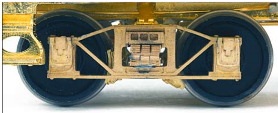
As with all of our models, everything that should open does, the underbody toolboxes on our N5 even has the proper locking hasps and pins secured by chains. Shown below is our PRR 2A-F1 type truck that is utilized on the N5 and several of the express version 'crew cars'.
