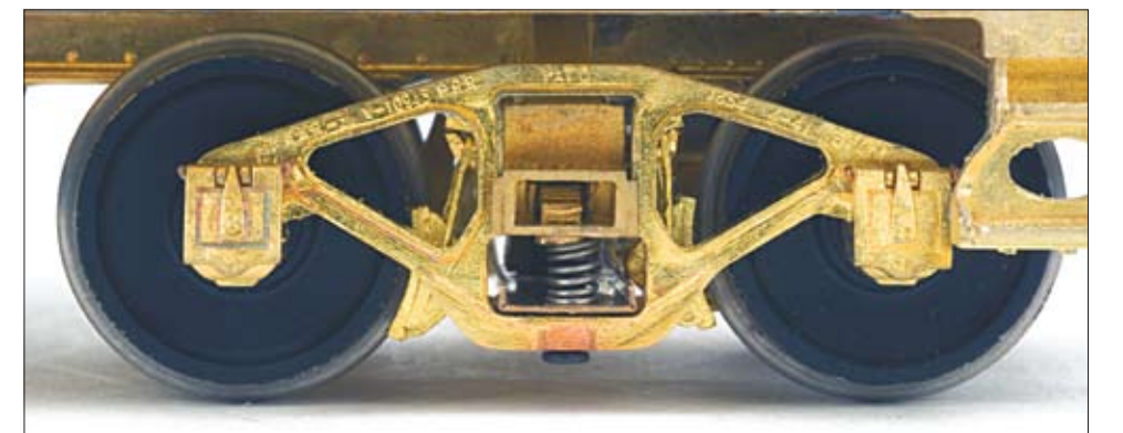
The interior above is an N5 arrangement as indicated by the position of the stove. Complete even with real wood flooring, no detail will be missed. Shown below is our PRR 2A-F5 type truck used on all N5b's and many N5 w/cp. Opening journal lids and ball-bearings are all standard.
